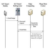
Figure 8. Sequence flow diagram between IoT device and edge computing.
