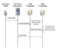
Figure 9. Sequence flow diagram between edge computing and other edge computing in inter/intra network area.
