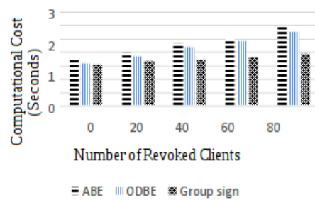
Figure 3. Comparison on client computation cost for file access among ABE, ODBE and group signature.
