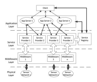
Figure 1. IoT architecture for context acquisition.
