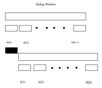
Figure 1. Sliding window and basic windows.
