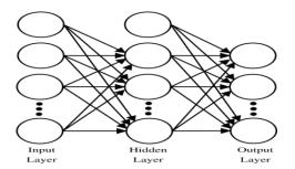
Figure 3. A Multi-Layer perceptron with one hidden layer.
