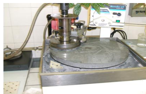
Figure 14. Grinding machine used for the commercial ferrite slab to obtain the 65 \mu\text{m} .
