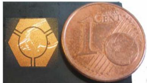
Figure 17. Photography of the circulator with shortened access lines.
