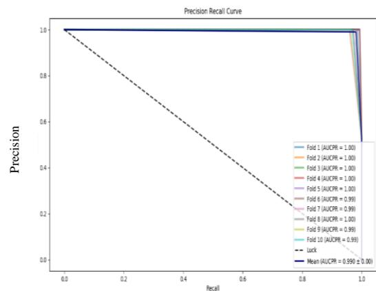
Figure 5. Precision-recall curve for multichannel LSTM.
