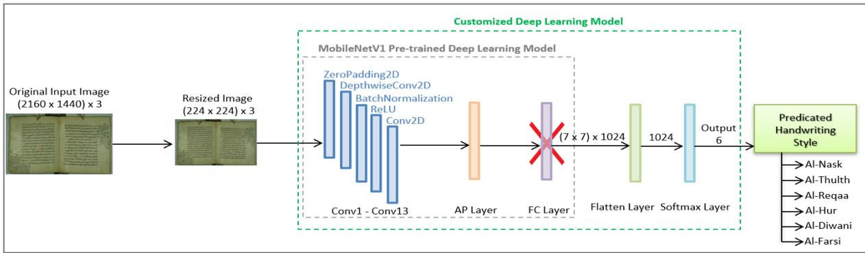
Figure 2. Architecture of the developed model.
