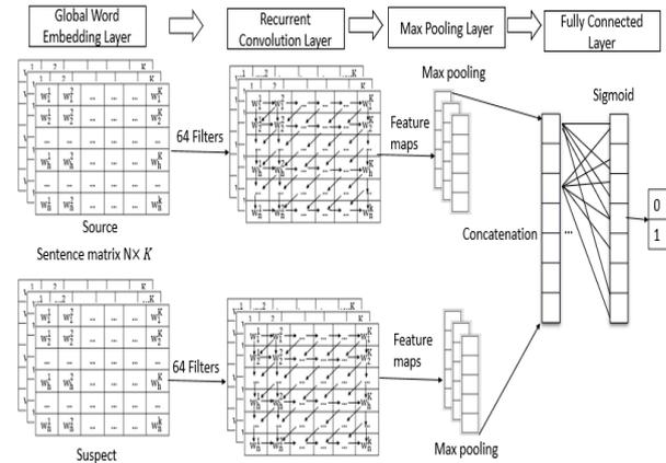
Figure 2. GloVe-RCNN model for Arabic paraphrase detection.
