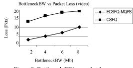
Figure 9. Bottleneck BW vs packet loss.
