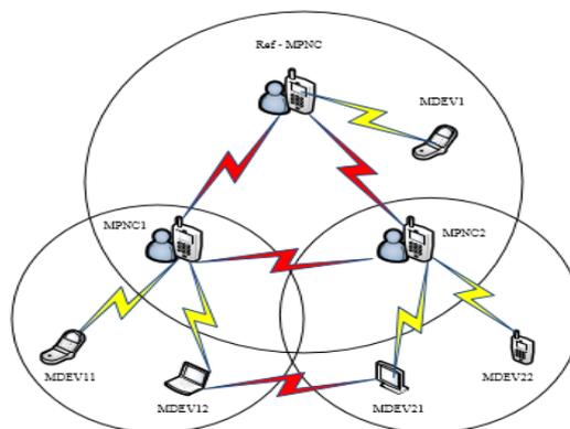
Figure 1. Two-hop IEEE 802.15.5 mesh network.
