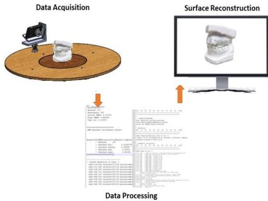
Figure 1. 3D reconstruction process steps.
