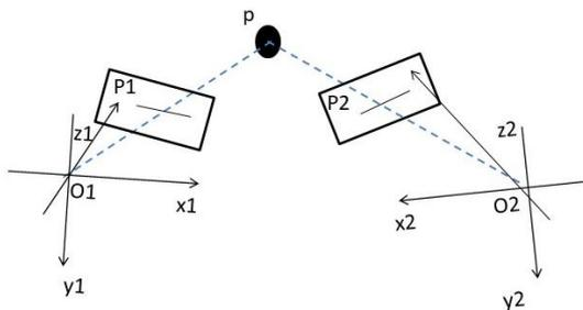
Figure 4. Acquiring 3D point from matched 2D points.
