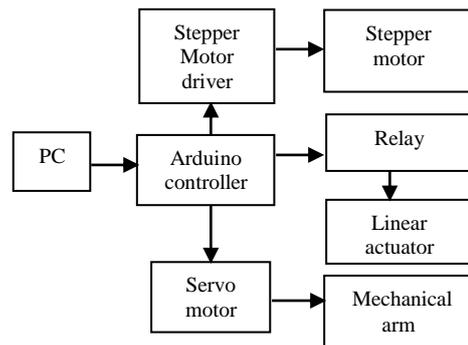
Figure 3. Hardware connections.
