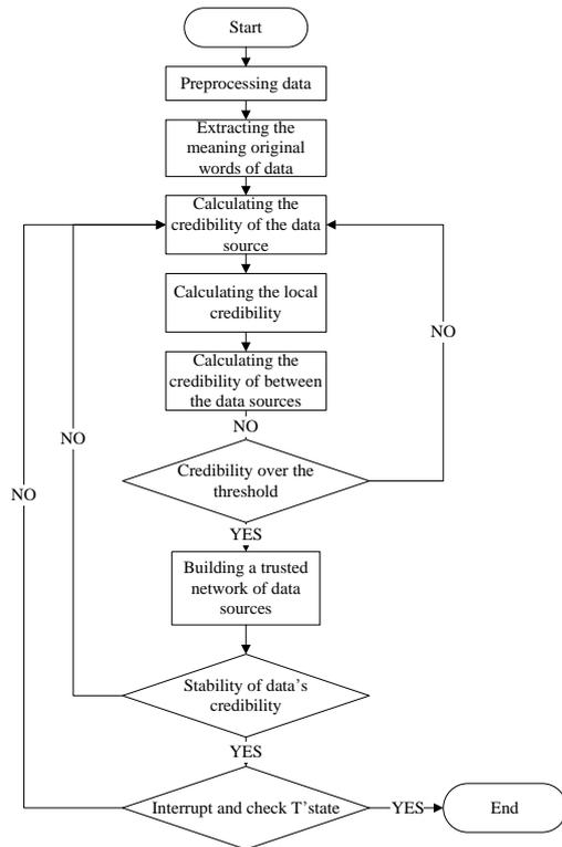
Figure 2. The program flow of the construction method of the trusted virtual network.
