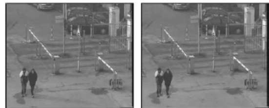
Figure 3. The benchmark "Campus" video sequence, image on the left corresponds to frame number 109 of the original video sequence, image on the right corresponds to the processed frame, cast shadow has been detected and removed.
