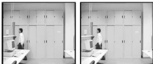
Figure 2. The benchmark "Laboratory" video sequence, image on the left corresponds to frame number 198 of the original video sequence, image on the right corresponds to the processed frame, cast shadow has been detected and removed.
