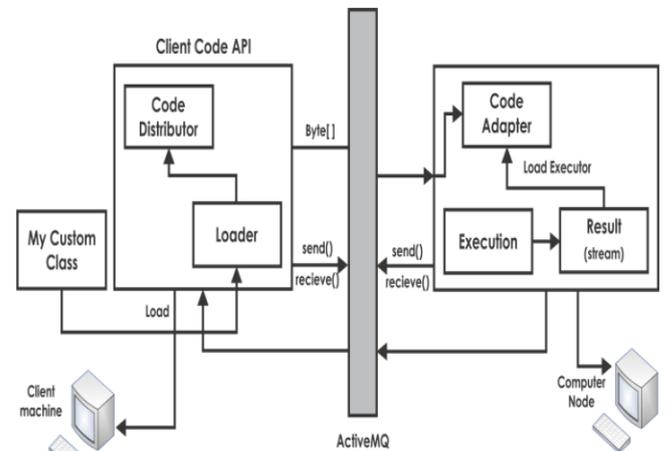
Figure 1. Component level diagram of code migrator/ execution.
