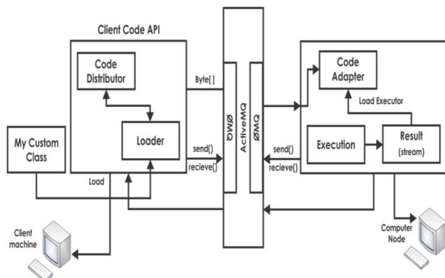
Figure 3. Code execution component of AA-JUMP.
