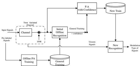
Figure 1. The overall block diagram of presented classifier.
