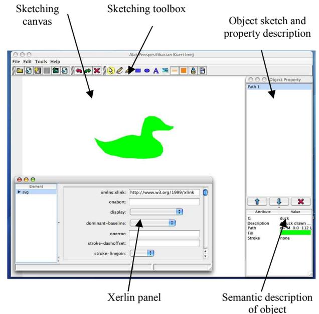
Figure 5. The query specification tool interface.
