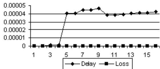
a. Delay and loss probabilities of real time cells using WRR.
