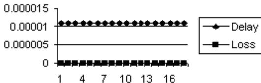
b. Delay and loss probabilities of non-real time cells using FIFO.
