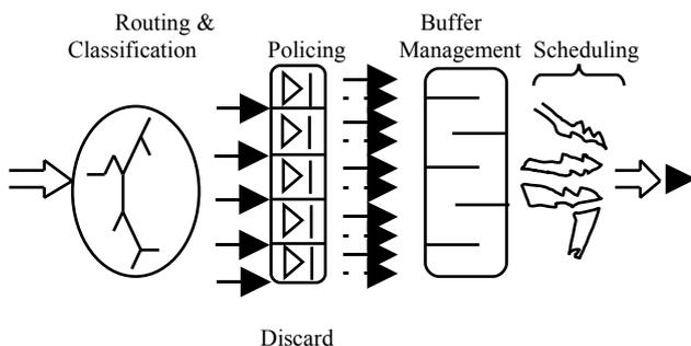
Figure 1. Combination of scheduling and buffer management in ATM traffic shaping.
