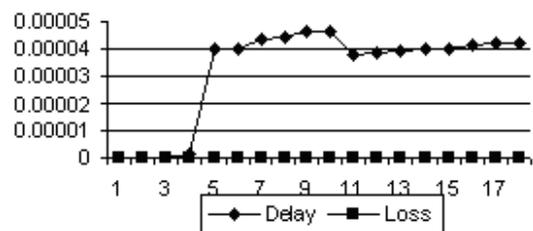
b. Delay and loss probabilities of non-real time cells using WRR.
