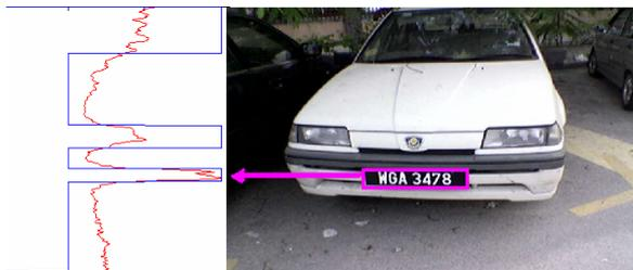
Figure 5. Horizontal projection of the edge image.
