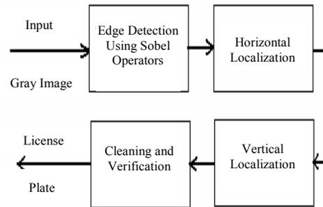
Figure 2. Plate extraction module.
