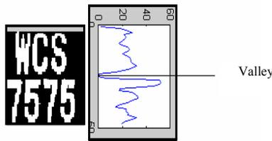
Figure 9. Horizontal projection of the plate.
