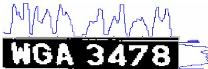
Figure 10 Horizontal and vertical projection of the license plate.
