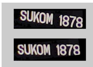
Figure 11 Skew angle correction.
