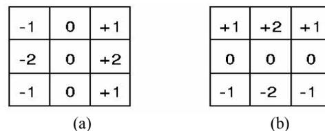
Figure 3. Sobel masks for edge detection, (a) Vertical, (b) Horizontal.
