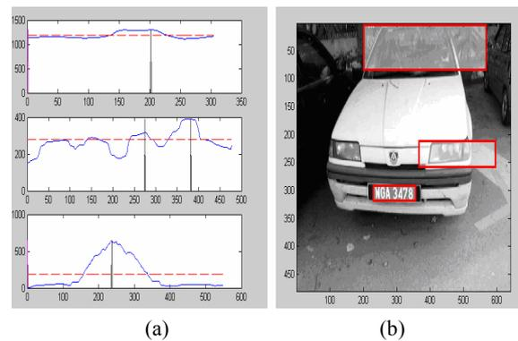
Figure 7. Example of vertical localization of the license plate.
