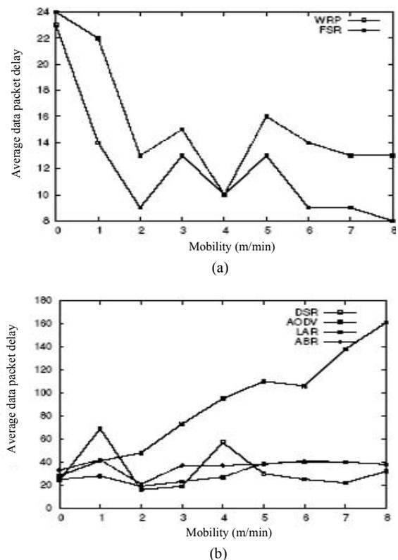
Figure 3. Average data packet transfer delay vs. mobility.
