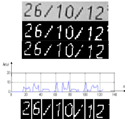
Figure 6. Segmentation of expiry date code. From top to down: Original image, binary image, thinned image, segmented expiry date numerals.
