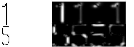
a) The segmented numeral. b) From left to right the LE feature map at four filter orientations ( \theta=0^\circ, \pi/4, \pi/2, 3\pi/4 ).
