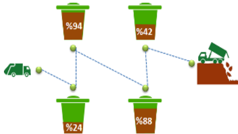
Figure 7. Unoptimized static route for waste collection.
