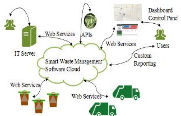
Figure 5. The principle of system operation.
