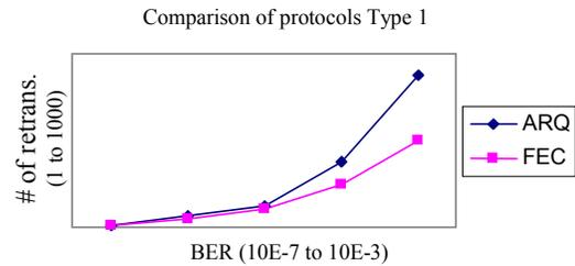
Figure 5. Comparison of ARQ versus FEC/ARQ with type 1.
