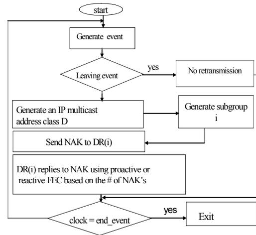
Figure 4. The abstract simulation model for the second part.
