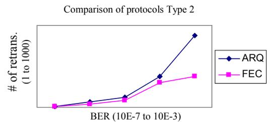
Figure 6. Comparison of ARQ versus FEC/ARQ with type 2.
