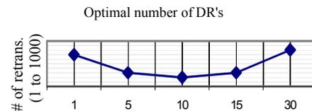
Figure 7. The number of DR's behavior with respect to the number of sender retransmissions is parabolic.
