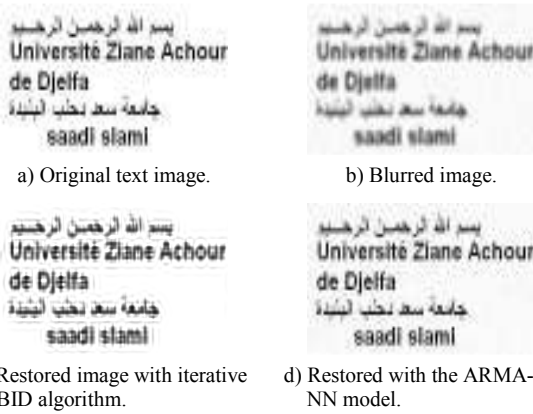
Figure 6. Comparison between the classical BID and our ARMA-NN model using a text image.
